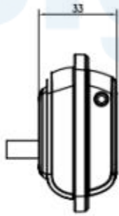
Embedded installation (mm)
